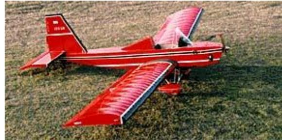
In the 303, visibility is always good. The cockpit is situated slightly forward of the wing's leading edge, giving you a clear view of what's above, around and below.
