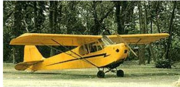
While your engine takes you up at a 900 to 1400 feet per minute climb, it also emits a relatively low noise level, effectively reduced by Lord mounts, tuned exhaust and geared reduction drive.
